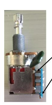
Leave a gap between the board and the pot base when soldering.
