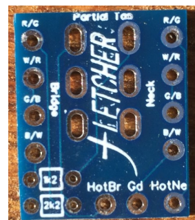
All PCB boards are marked for FletcherPickups wire colours.
